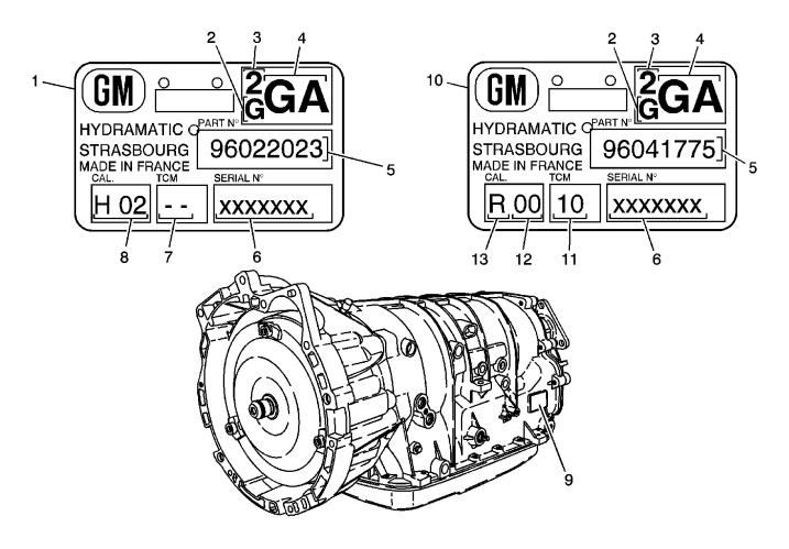
**Important:** Always check the transmission ID before performing internal repairs.
