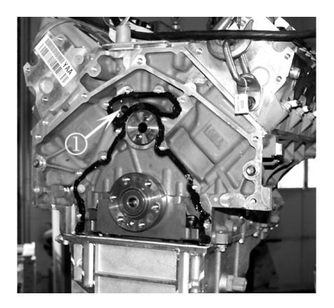
**Important:** Clean any residual oil from the block and cover before applying the sealant in the next step.
