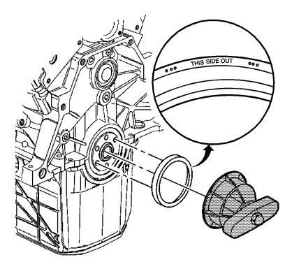
**Notice:** Do not apply or use any oil lubrication on the crankshaft rear oil seal or the seal installer. Do not touch the sealing lip of the oil seal once the protective sleeve is removed. Doing so will damage or deform the seal.
