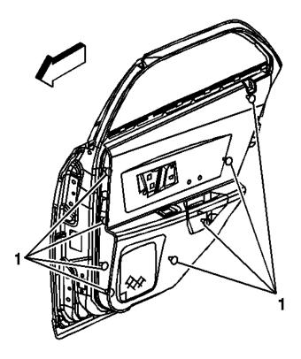
3. Install the door trim panel by applying pressure around the door trim panel to secure the retainers (1) to the door.
