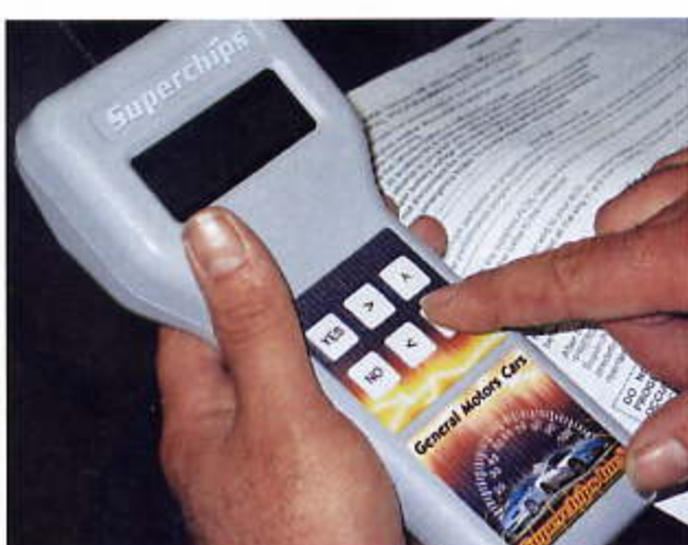
Next, we connected the Superchips tuner that was supplied with the blower kit, and we loaded the program. With this done we replaced the Audio fuse and then disconnected the battery as per the instruction manual.
