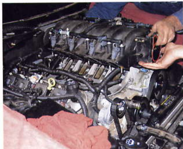
With the fuel lines disconnected, the intake was unbolted and carefully removed.
