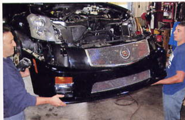
Once the cover was off the engine, we removed the radiator mask, the lower splash pan and the front fascia, all of which unbolted in a matter of minutes.
