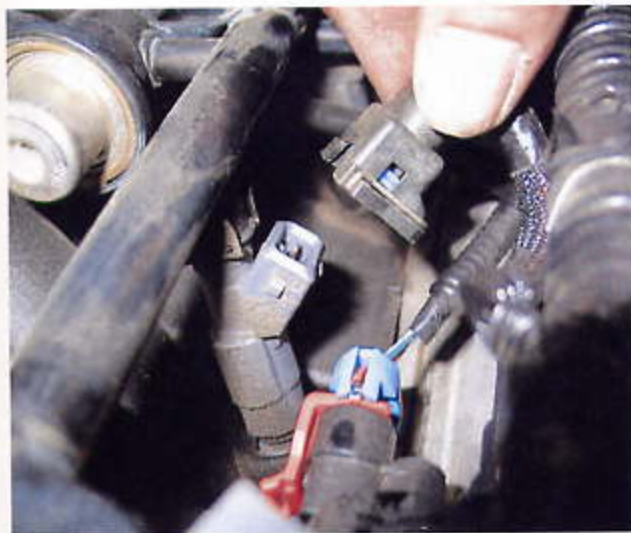
We then unplugged the eight 28.5-lb injectors (shown) along with the electronic throttle control (ETC), the throttle position sensor, both coil packs, and the MAP.
