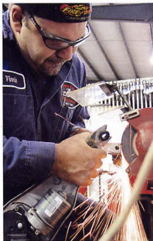
Vinnie then removed the windshield wiper arms along with the wiper motor assembly. It is necessary to grind a small portion of the wiper arm so it will clear the blower drive system.
