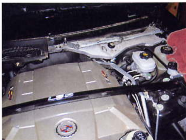
Vinnie then removed the windshield wiper arms along with the wiper motor assembly. It is necessary to grind a small portion of the wiper arm so it will clear the blower drive system.
