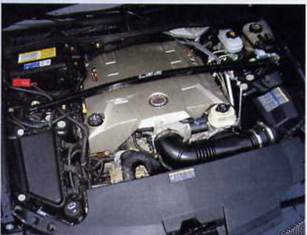
Stock CTS-V LS6 is rated at 400 horsepower and 395 lb-ft of torque. Once supercharged, the LS6 pumped out 451 horsepower and 438 lb-ft of torque at the wheels.
