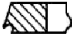
This is a side view of a second compression ring having a Napier profile face. Drawing: Author
