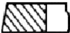
This is a side view of the scraper face on a typical second compression ring. Drawing: Author.
