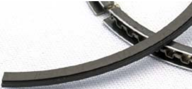
[Above] The unique scraper face of the Napier profile, second compression ring, shown upside down for demonstration purposes, is clearly evident here. Image: Author. [ Click Image for Larger View ]
