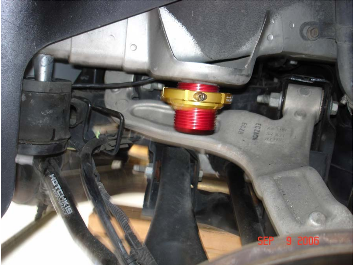
13. Install lower mount per GC sketch.
